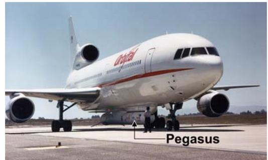
"The aircraft eliminates the need for a large first stage on the rocket," explains Surber. "Because *Stargazer* can be used for many missions, it becomes a re-useable first stage and makes the launch system cheaper in the long run." (To take advantage of this inexpensive launch system, GALEX designers had to make their spacecraft weigh less than 1000 lbs-the most a Pegasus can carry.)
